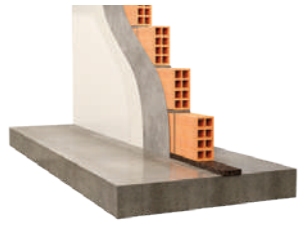
Internal partitions Masonry wall and slab discontinuity
