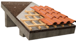
Roofs Pitched roof with roof membrane
